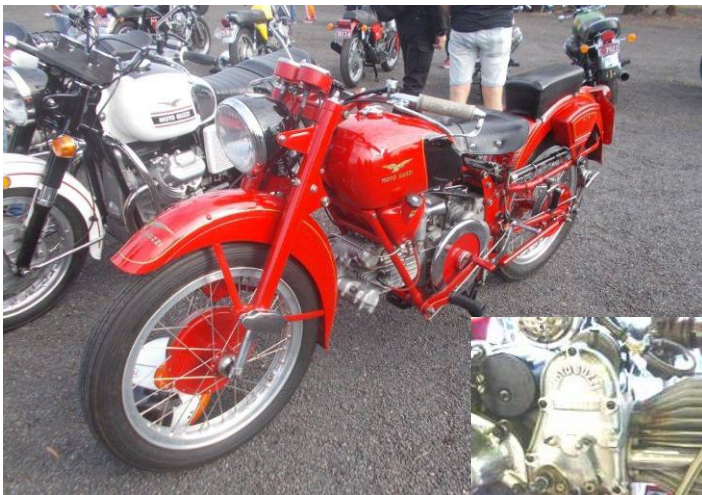
▲ Another iconic Italian bike was the Moto Guzzi with it's big horizontal cylinder and exposed flywheel whizzing around your left ankle .
