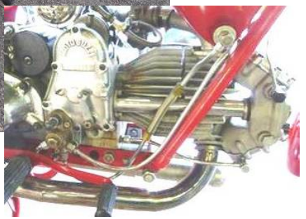
▲ Another iconic Italian bike was the Moto Guzzi with it's big horizontal cylinder and exposed flywheel whizzing around your left ankle .
