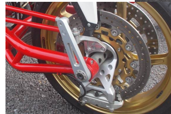
◀ The front wheel is suspended on a swinging arm frame in place of sliding forks while the steering pivot is inside the hub rather than the frames headstock . Different but not better seems to be the verdict !
