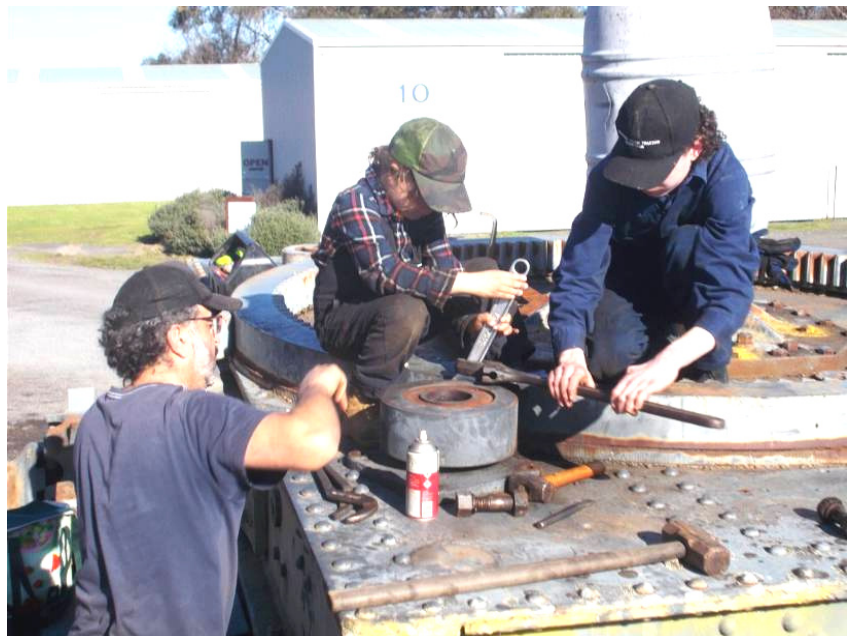
Spiros , Koby and Greg unbolting the stuck roller. Steam Supreme June 2024 .
