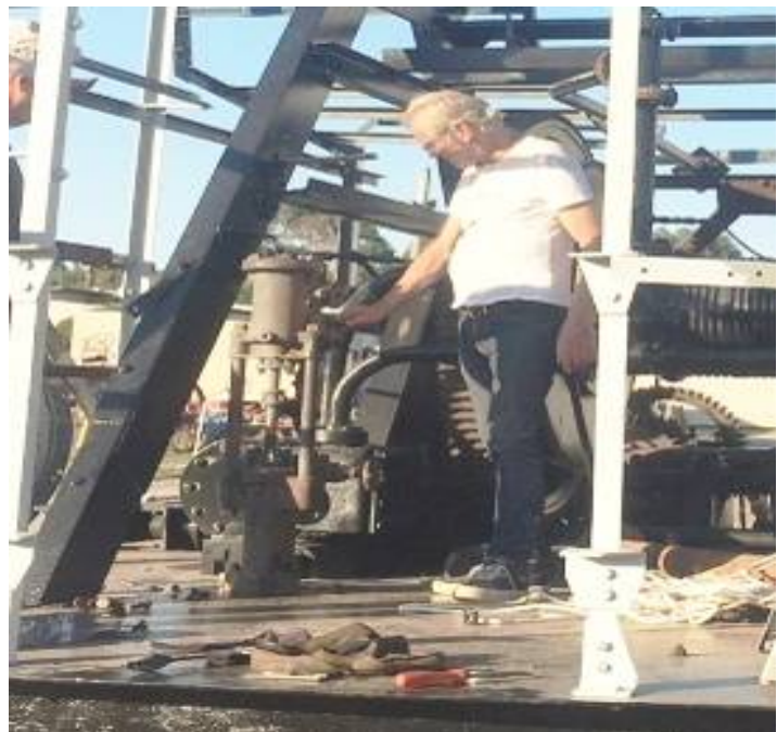
John Mills fathoming out the feedwater plumbing between the pump and heater. The Weir pump is free and appears to be complete and in good condition .
