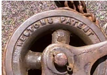
↑ Above the endless chain sees light of day after 25 years . Note the 13 metres of tangled chain WESTONS PATENT is clearly cast into the differential pulley . The other writing says TESTED TO 1 TON
