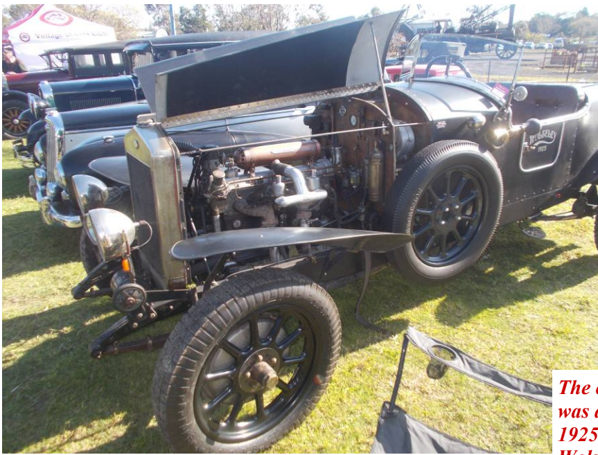
The 16/ 65 single overhead cam engine is 65 brake horsepower at 4,400 rpm in twin carby form .
