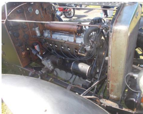
The 16/ 65 single overhead cam engine is 65 brake horsepower at 4,400 rpm in twin carby form .
