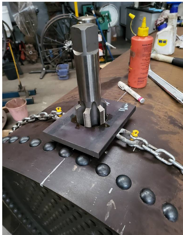
The tap we had made using the pre tapped guide to align it.
