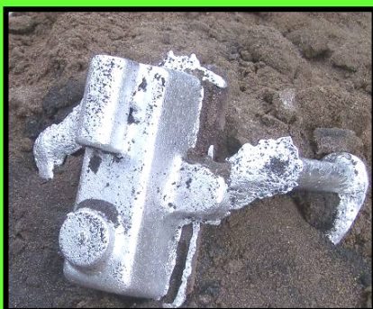
Lets do our own Castings Stuart tank headlight bracket
