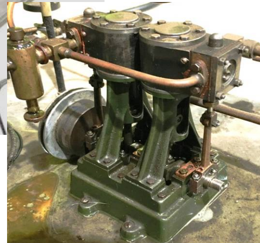
A closer up of the Twin cylinder engine basically 2 singles on a common base
