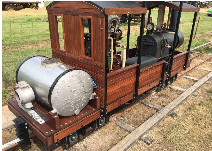
The driver sits 1/2 way along the loco behind a conventional horizontal water tube boiler as you might find in a portable or traction engine . He is high enough to get a good view over it
