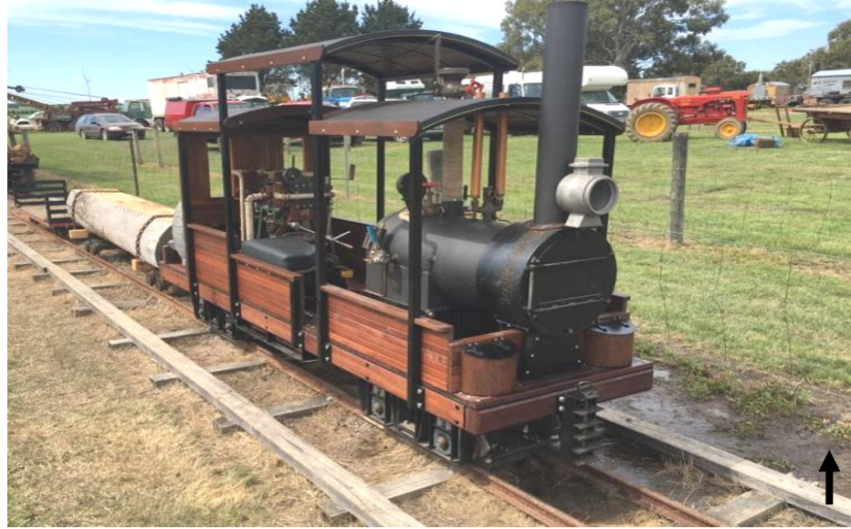
The driver sits 1/2 way along the loco behind a conventional horizontal water tube boiler as you might find in a portable or traction engine . He is high enough to get a good view over it
