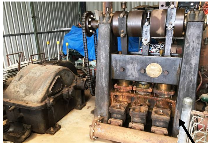
A closer up view of the Kelly and Lewis triple flow positive displacement pump of 15,000 gallons per hour at 55 rpm. To its left is it's Richardson's reduction drive gearbox which in turn is driven by 6 inch wide flat belt from the 28 hp Ronaldson Tippet Diesel
