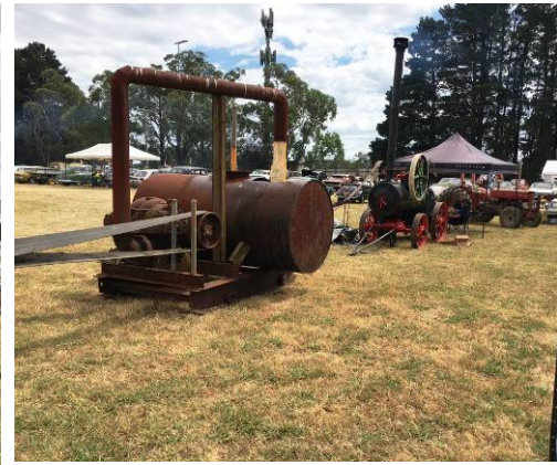
Colemans Buffalo Pitts traction engine was displayed driving a flood irrigation pump through a long belt
