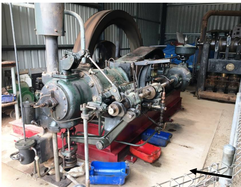
A closer up view of the Kelly and Lewis triple flow positive displacement pump of 15,000 gallons per hour at 55 rpm. To its left is it's Richardson's reduction drive gearbox which in turn is driven by 6 inch wide flat belt from the 28 hp Ronaldson Tippet Diesel
