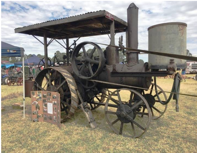
Colemans Buffalo Pitts traction engine was displayed driving a flood irrigation pump through a long belt
