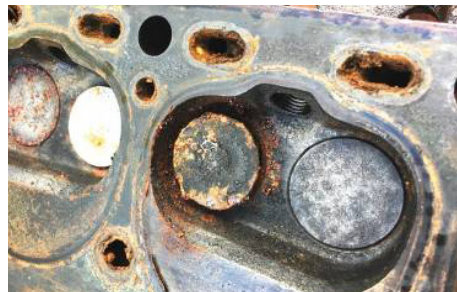
Ruined Valves and pitted seats
