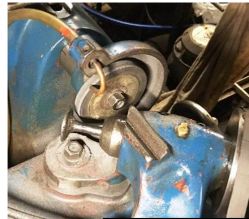
Refacing the valves
