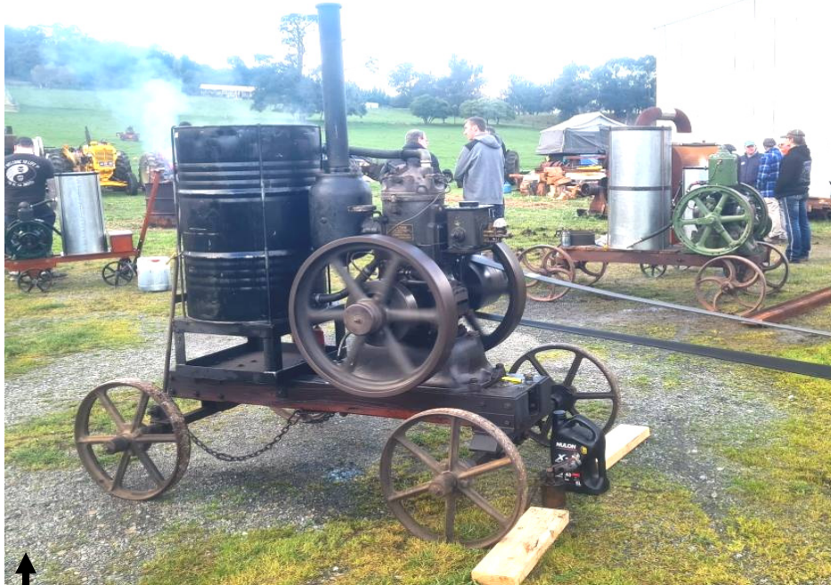
Amongst the visiting engines lined up outside was this Petter S Crude Oil 2 stroke Engine . Note various others in the background being admired.
