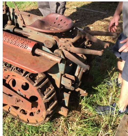
Details of the implement linkage and track joints
