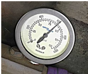
← By the end of the day we had all the tubes in and had it up to 100 psi pressure with water from the main .
