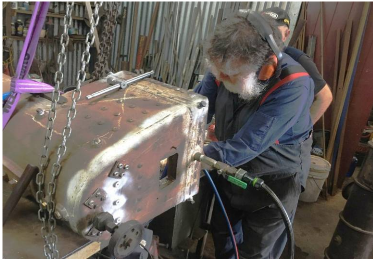
← By the end of the day we had all the tubes in and had it up to 100 psi pressure with water from the main .
