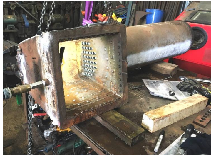
← By the end of the day we had all the tubes in and had it up to 100 psi pressure with water from the main .
